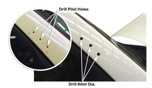
Secure the upper mounting bracket (Item 3) to the A-pillar with three self-tapping screws (Item 5).
