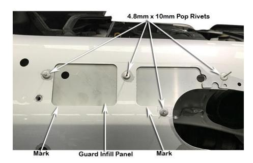
Apply Sikaflex 227 to the outer edges and centre of the guard infill panel (item 14) as shown, install the infill panel to the guard panel, install all 4 pop rivets (item 15).
