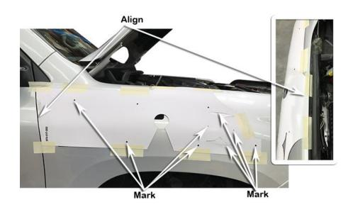
Drill a pilot hole for each of the marked positions.
