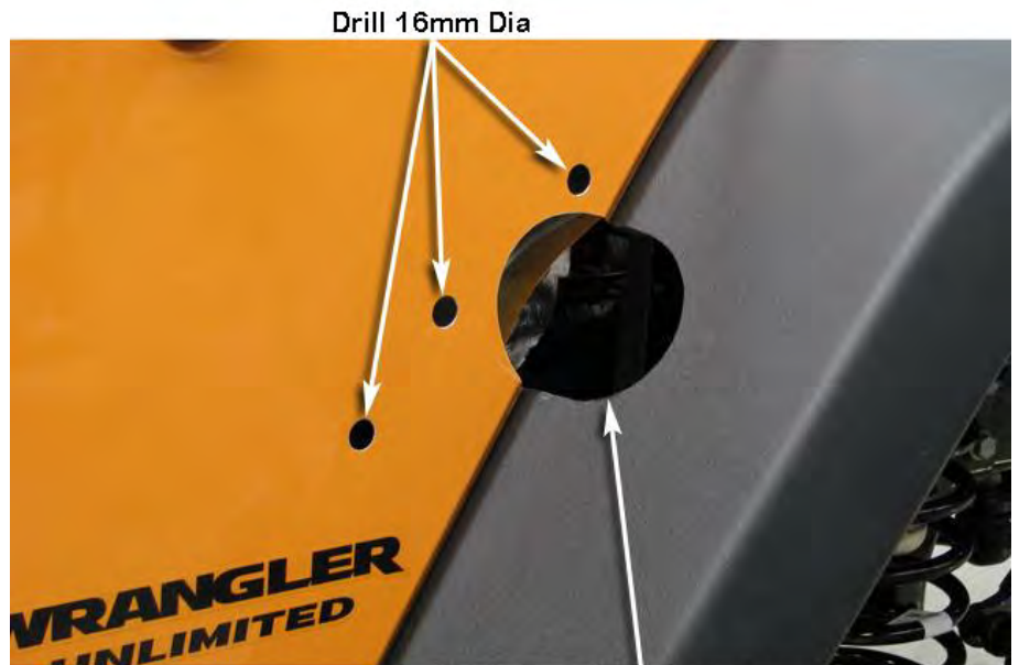
Cut Using Air Body Saw
