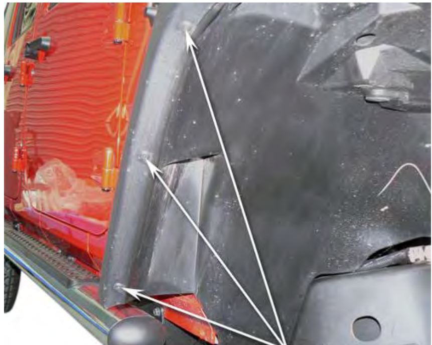
Remove Plastic Pop Rivets
