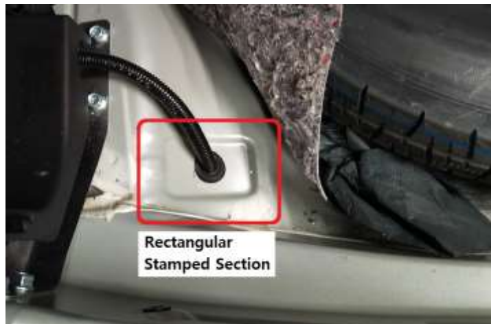
Figure 1: Location of rectangular stamped section (pre-drilled & harness installed)
