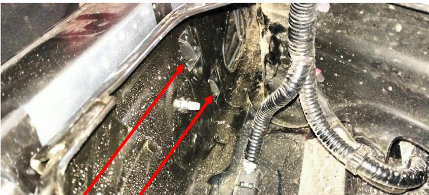
Disengage the clips to separate the step cover from the bumper body.
