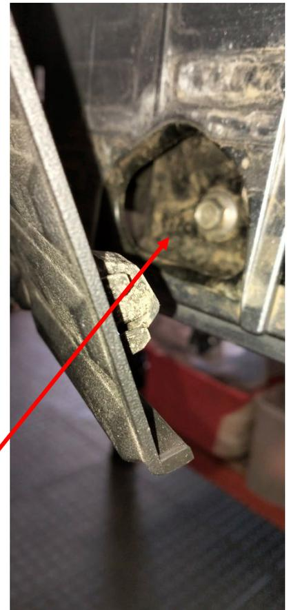
Remove bolts from bumper bar mounts.
