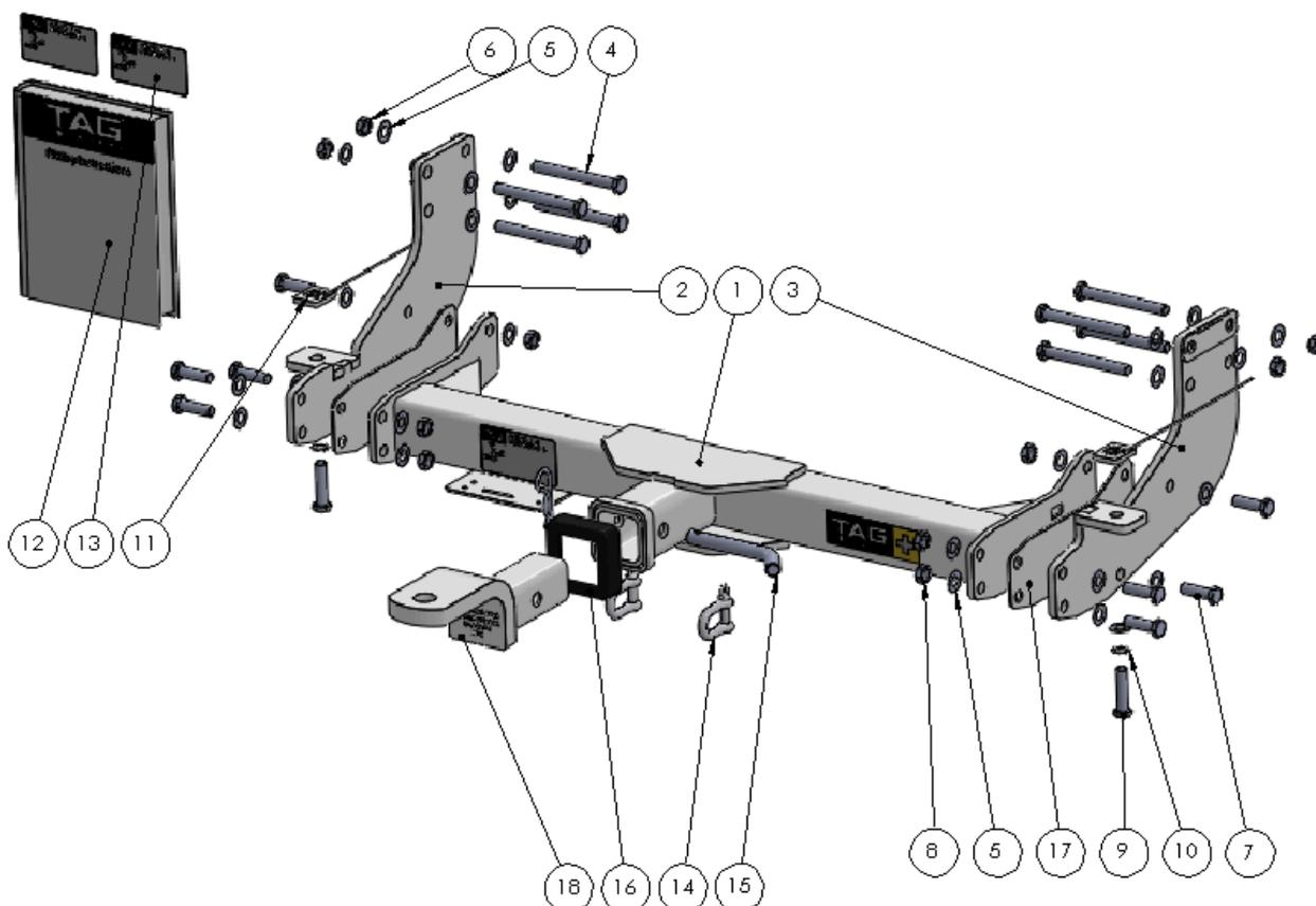
Tools Required: Spanners, Sockets, Screwdriver, Torque wrench
